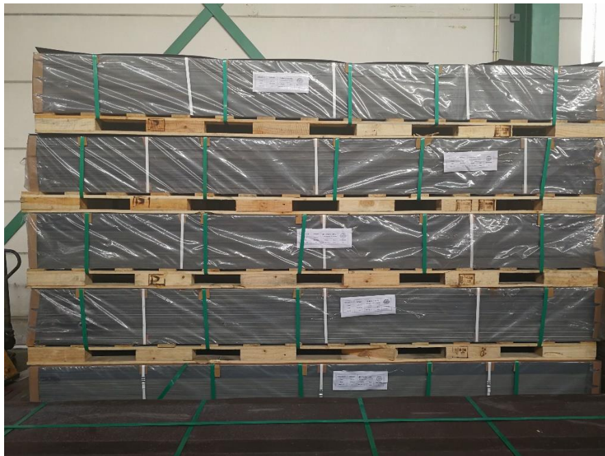
Figure 5: Correct handling, storing and transportation of JD Basic COMPACT
